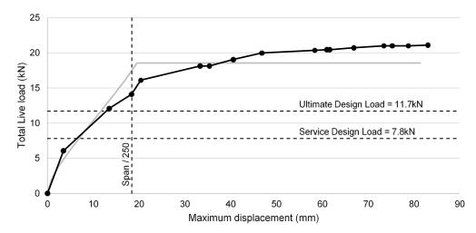
Figure 6. Load vs. displacement plot of prototype test, experimental results in black and predicted in grey.
