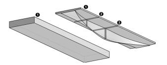
Figure 2. Overview of the design methodology: as opposed to the design of a prismatic slab where one section is designed for the maximum loading conditions, multiple sections are shaped according to the required capacity along the length of the slab.
